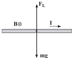
$$F_L = mg \quad \text{ή} \quad BI\ell = mg \quad \text{ή} \quad B = \frac{mg}{I\ell} \quad \text{ή}$$
